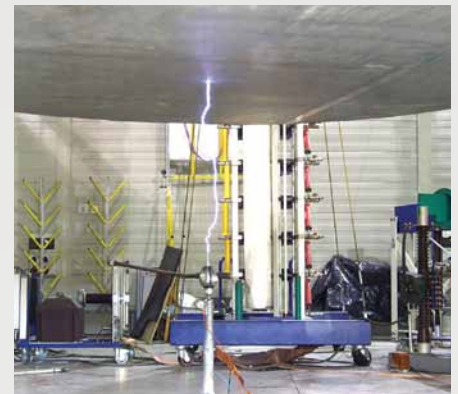
Testing of the Stormaster Terminal: ITE HV Laboratory, Europe
